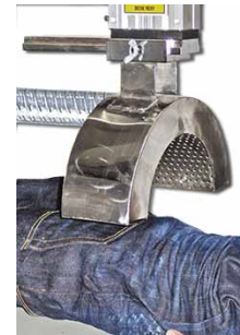
3D crinkle operation for smooth results
