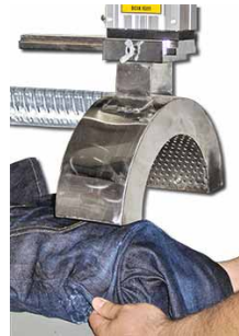
Normal crinkle operation for sharp creases
