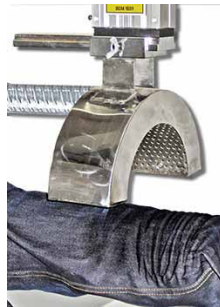
Normal crinkle operation for sharp creases
